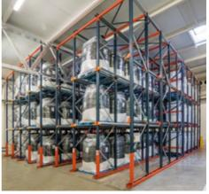
CAN BE USED WITH EITHER LIFO (LAST IN, FIRST OUT) OR FIFO (FIRST IN, FIRST OUT) WITH BATCHES WHEN THERE ARE MORE THAN THREE LANES PER SKU.
