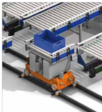
Details of a shuttle (1).
