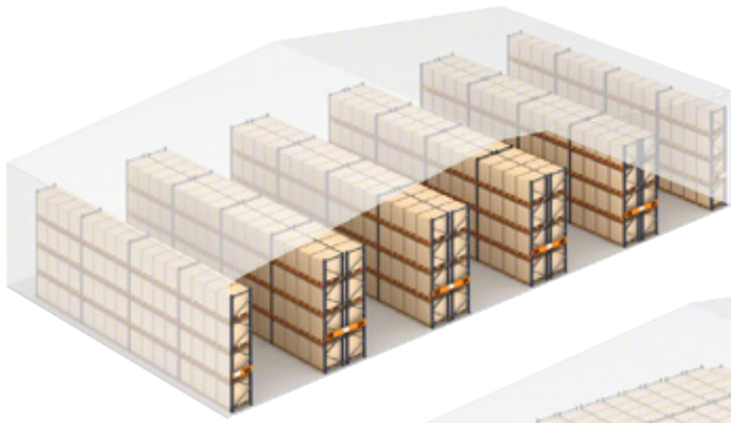
Warehouse using conventional pallet storage.
