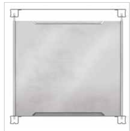
Detail of attachment to upper and lower shelf.
